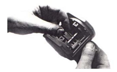
**8.** Now take a flat head screwdriver and pry off the top of the Pilot Slide (#70) Slide out the Bottom part of the Pilot Slide (#69) from under the steel shaft.
