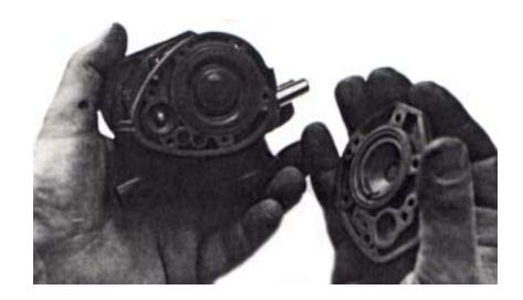
2. Now you can replace the diaphragms in this side of the pulsator 1 large 1 small and the 2 tiny sealing rings. Take care to make sure the replaced parts are properly seated, replace the cover and install the screws. Repeat this procedure on the other side of the pulsator. This completes the installation of the economy replacement kit.
