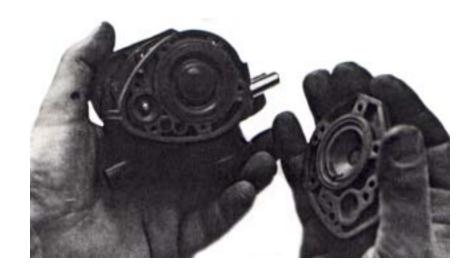
**4.** Now you can remove the diaphragms in both side of the pulsator 2 large 2 small and the 4 tiny sealing rings. Once all the diaphragms and sealing rings are removed proceed to step 5.
