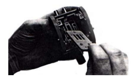
**10.** Seperate the Base Plate Gasket (#58) from the Base Plate (#57). Install the new Gasket and Base Plate back into the pulsator.
