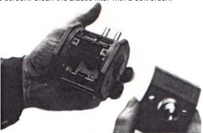
**6.** To change the slide, take a flat head screwdriver and pry off the slide cover (#66)
