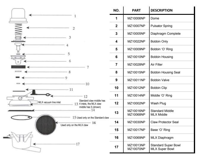
Note: The MLX style claw has a separate vacuum line, so there are 5 inlets on the middle, a bleed-hole on the base under the rubber hook and it uses the MLX diaphragm between the base and middle. The Standard style claw uses the Base O-Ring between the middle and base.
