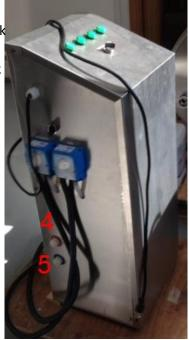
As soon as you finish with water connection and you plug in the power you can you use the switch located on the top of the panel to start washing.
