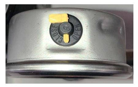
Finally, install the muffler onto the outlet of the pump.
